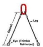
Sling – an assembly which connects the load to the lifting equipment
