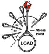
If the angle is less than 120°, you must adjust its Choker Hitch Working Load Limit by the appropriate choke factor from this table.
