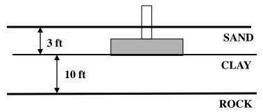
Solution: Since the water can't drain into rock the longest path is into the sand on the top, so the water molecule at the bottom of the clay layer will have to travel the 10 ft to the sandy soil.  $\mathbf{H} = \mathbf{10}$  ft.
