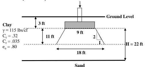
Step 1: Write down the consolidation settlement equation:  $\Delta H = H \times Cr/(1 + e_o) \times \log ((p'_o + \Delta p1)/(p'_o) + H \times Cc/(1 + e_o) \times \log ((p'_c + \Delta p2)/(p'_c))$
